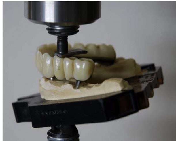
Fig. 6–7. Detail of compression test 1 with interposition of a lead laminate between the punch and the denture.
