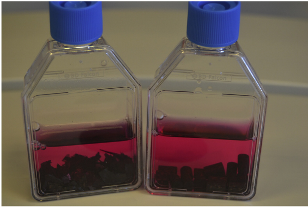
Fig. 1. Extraction flasks containing fragmented samples (on the left) and intact samples (on the right).
