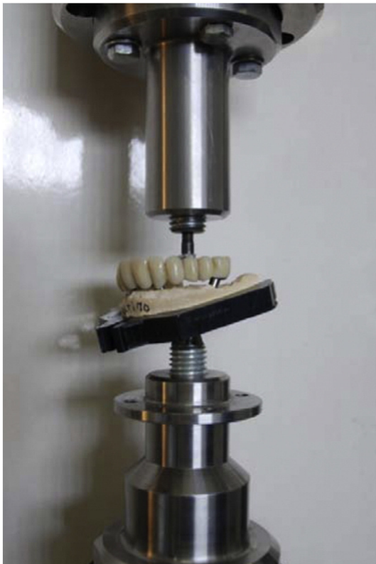
Fig. 6–7. Detail of compression test 1 with interposition of a lead laminate between the punch and the denture.
